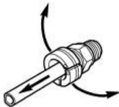
Fig. 91: Oil Cooler Line Quick Connect Fitting - Disassembly Courtesy of CHRYSLER LLC
