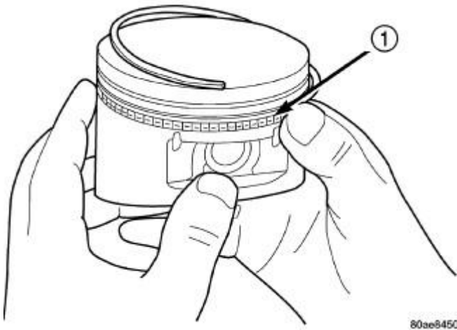
Fig. 222: SIDE RAIL - INSTALLATION Courtesy of CHRYSLER LLC
