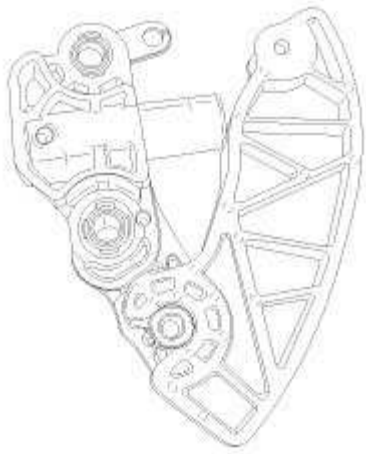
Fig. 457: Timing Chain Tensioner Arm Courtesy of CHRYSLER GROUP, LLC
