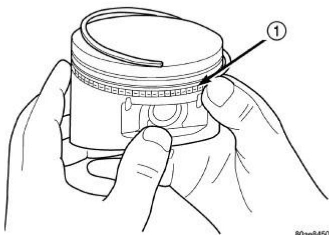
Fig. 480: Removing/Installing Piston Ring Side Rail Courtesy of CHRYSLER GROUP, LLC
