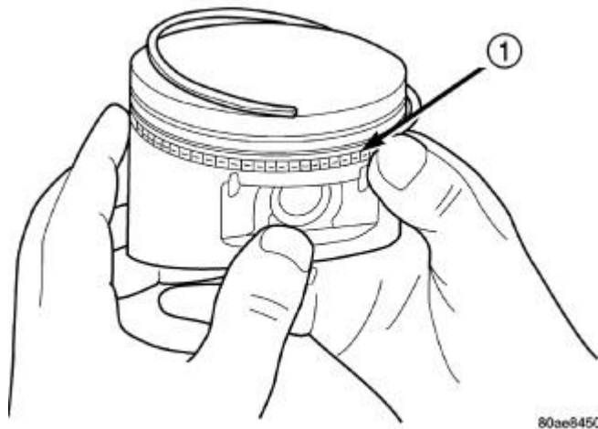
Fig. 221: SIDE RAIL - INSTALLATION Courtesy of CHRYSLER LLC
