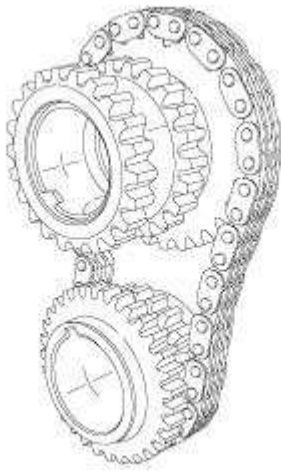
Fig. 716: Primary Chain, Idler Sprocket & Crankshaft Sprocket Courtesy of CHRYSLER GROUP, LLC
