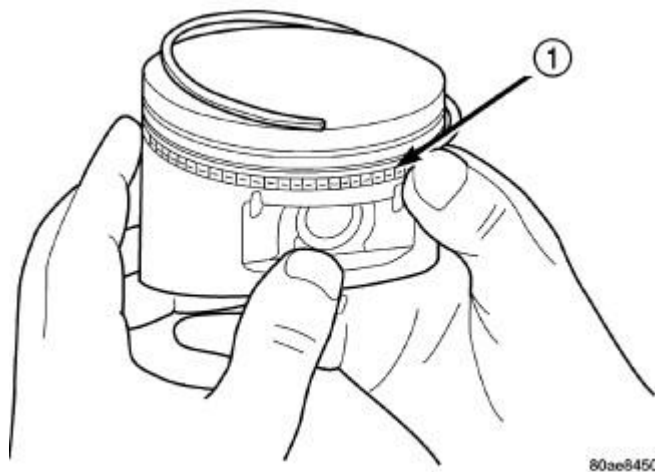
Fig. 478: Removing/Installing Piston Ring Side Rail Courtesy of CHRYSLER GROUP, LLC
